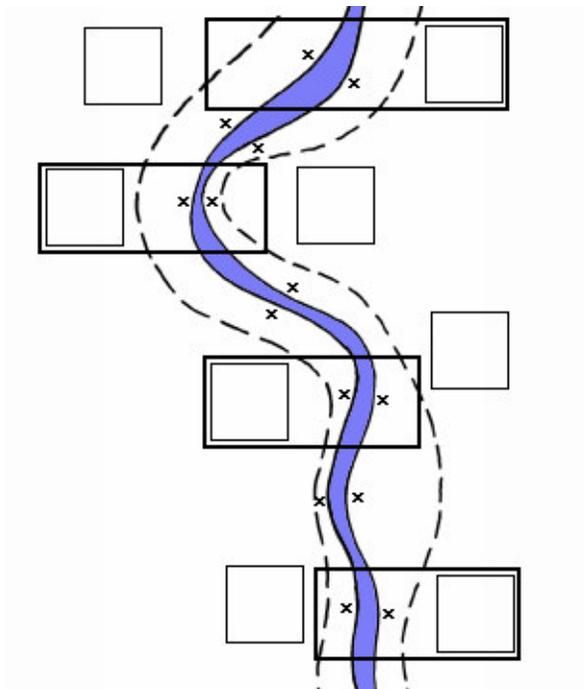
Fig. 1. Generalised layout of experimental plots at Native Cat Flat and Cowombat Flat. Squares are monitoring plots, bold lines are fences, the dashed line is the limit of direct riparian (streamside) influence. Crosses represent points on the streambanks permanently marked with star posts for the stream transects.
